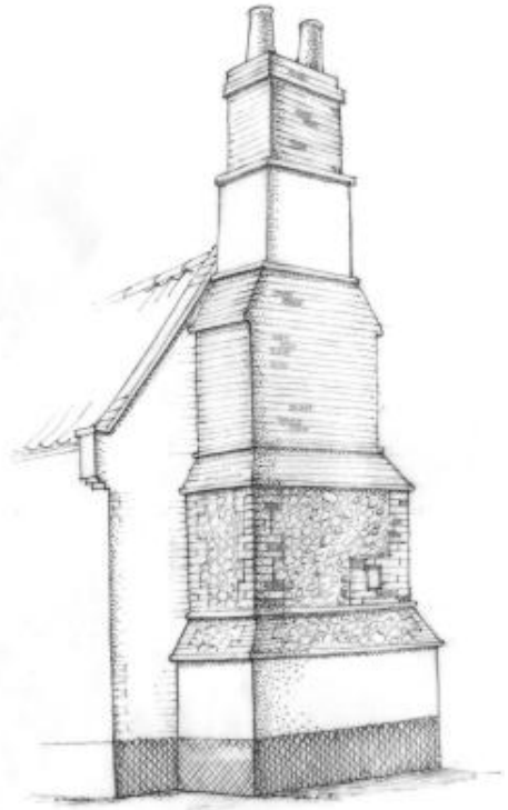
External chimney stacks are rare - where they do exist they are made a major visual feature as in this 17th century example at Cley-next-the-Sea.
