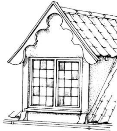
Gabled type (usually with plain bargeboards) of 17th - 20th centuries.
