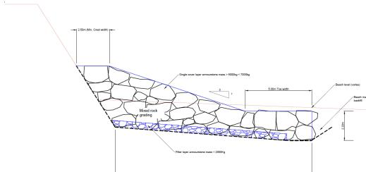
Figure 3. Cross section through rock revetment
