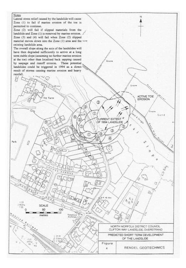
Figure 4 - Projected Development of Landslide
