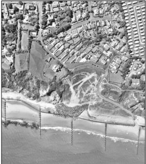
The top left photograph is shows Clifton way in 1986 before the major failure occurred. The top right photo is from 1994 and shows the extent of the failure at that time. The photo on the left was taken in 2000, approximately 5 years after the site was stabilised. The rock armour is clearly visable at the toe of the slide and many of the surface drains can also be seen.
