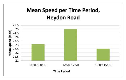
2. Speed survey using data from the SAM speed indicator November 2016
