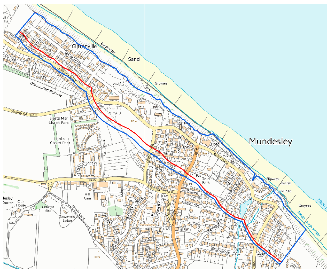
Figure 2: SCAPE model erosion extents. Do Nothing outline is shown in blue and the SMP6 scenario outline is shown in red.
