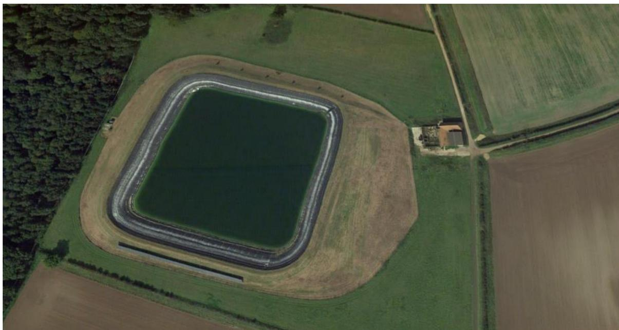
**Figure 3.9: Reservoir at Holkham (total area approx 5 ha), showing grassed embankments and rubber lining.**
