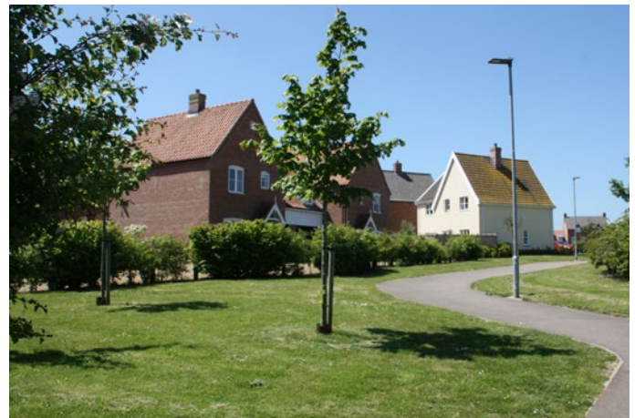
Figure 46: Local examples of street lighting with appropriate distance from the dwellings in order to avoid causing disturbance to the residents and light pollution.
