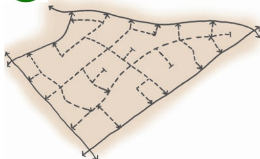
Figure 44: A connected layout, with some cul-de-sacs, balances sustainability and security aims in a walkable neighbourhood.
