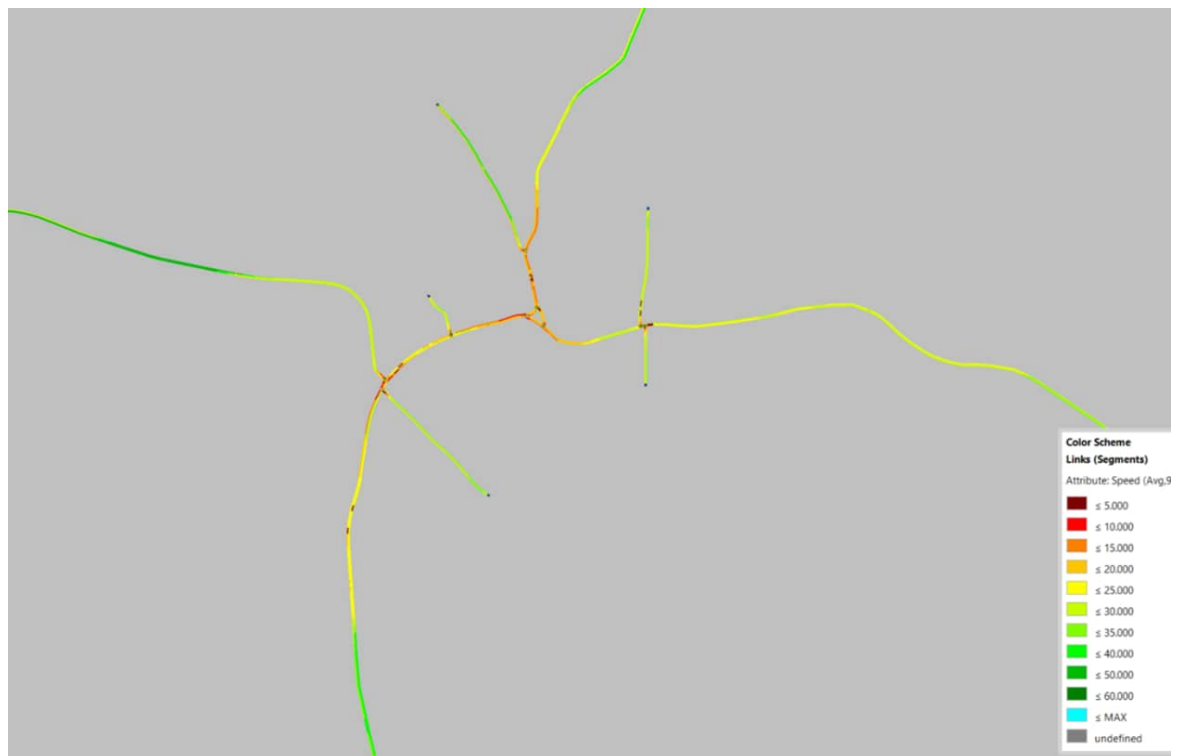
Figure 10 – AM Peak Hour Speed Plot
