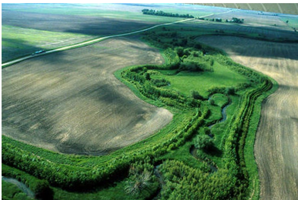
Figure 3.3 Aerial view of a riparian buffer strip (Source: Iowa State University Forestry Department, 2016).
